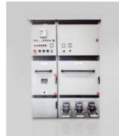
The Shore Connection Panel typically consists of a circuit breaker panel and a connector panel, which can vary in number and size depending on the current requirements and the connection system in place. The electrical characteristics of the SCP can reach values of 12 kV-50kA-2000A. The sockets are installed in the connector panel to ensure easy access while preserving the electrical requirements, and providing protection against potential internal arcs.
